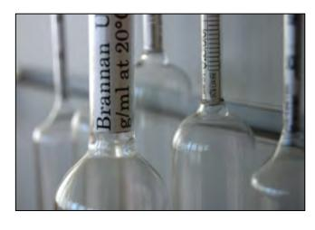
(or, exceptionally 15°C). For use in tropical countries, ISO 387 proposes that hydrometers be adjusted at a higher reference temperature, 27°C (as opposed to the previously used high adjustment of 84°F).
