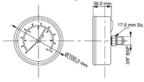
100mm Dial Pressure Gauge 1/2" BSP - Bottom Entry
