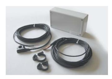
Nuaire AIREMISER-CM automatic fan controller comprise of a main controller with the optional choice of either or both current and temperature sensors which detects when a cooker or shower is in use. This enables the AIREMISER-CM to automatically turn on an extract fan or boost a central ventilation system.
