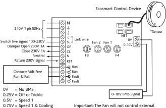
Heating/cooling equipment, will only provide ON/OFF Signal
