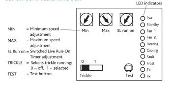
The Ecosmart control module has the following two options fitted as standard.
