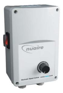
The electronic speed controllers provide infinitely variable speed control from preset minimum to maximum. All models feature a boost start function, which applies maximum power to the motor for 10 seconds to prevent motor stalling before returning to selected speed.
