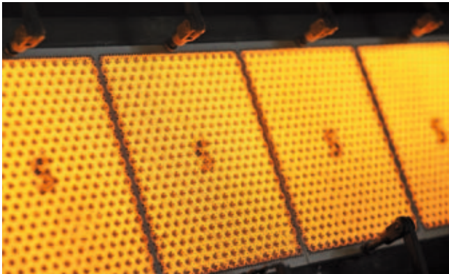
Schwank ceramic burner tiles subject to life-cycle tests.
