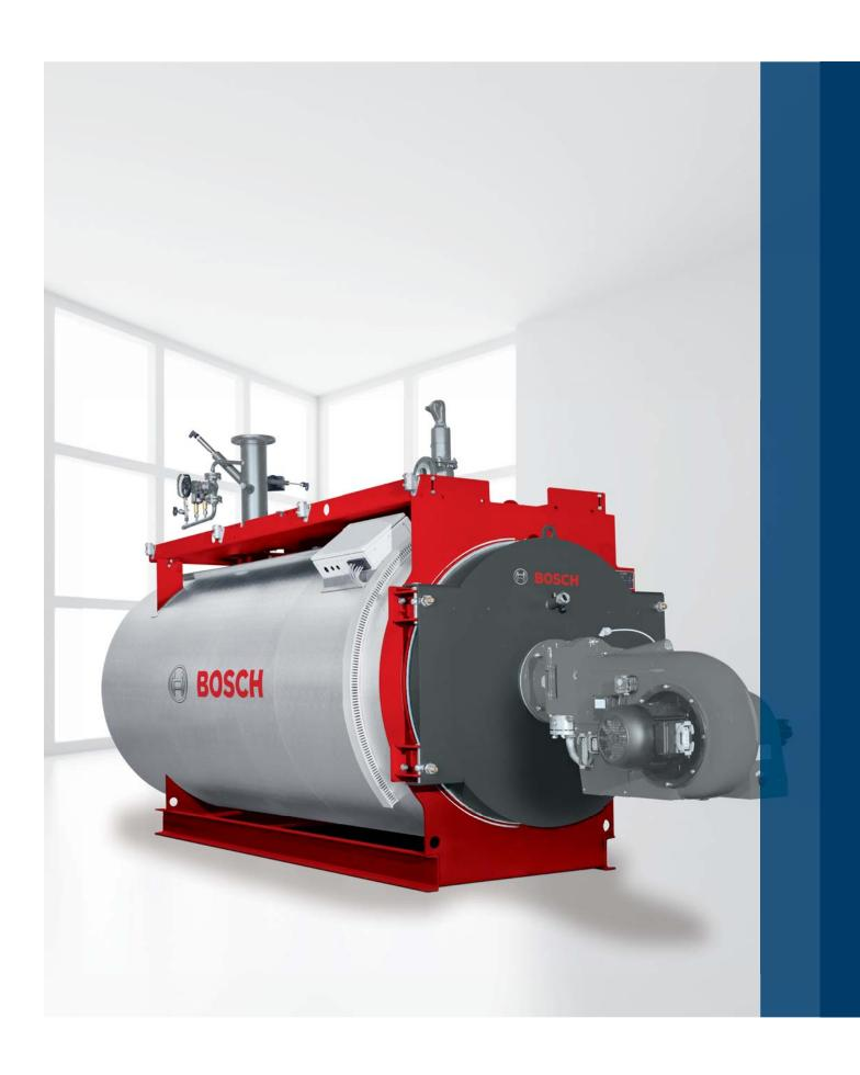
The inserted flame tube ends in an inner, waterflushed smoke gas reversing chamber, which leads into the first smoke tube pass. The first smoke tube pass and second smoke tube pass are free of flow components. The functional round design ensures optimal pressure resistance. Furnace, water chamber volume, radiant and convective heating surfaces are perfectly dimensioned and matched to each other.
