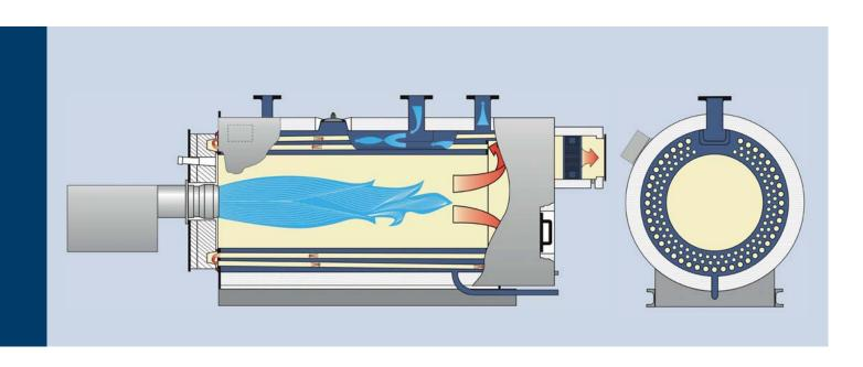
The UNIMAT hot water UT-M boiler is offered as a fully operational unit including operating equipment\*. The high quality equipment includes the boiler pressure vessel, burner unit, flue gas heat exchanger or condensing heat exchanger and the control and safety technology, which is already wired with the integrated terminal box. Pre-assembled, plug-in and coded cable bundles simplify the electrical wiring installation between the boiler control cabinet and the terminal box.
