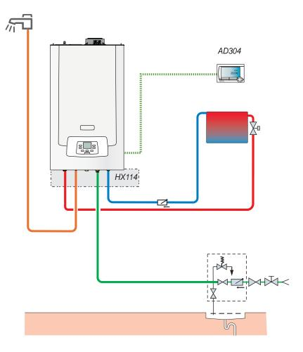
One direct circuit to radiator, with instantenious domestic hot water production and connected thermostat
