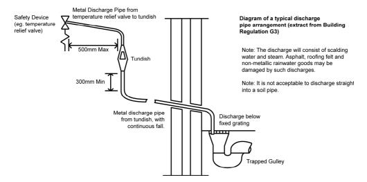
General guidance is provide by the above diagram extracted from the G3 Building Regulation Guidance.
