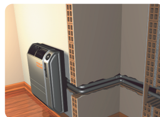
Wall separate pipes
