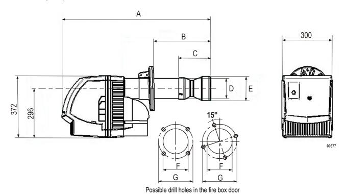
**1** Leave a minimum space of 1.00 m behind the burner, free of any obstacles to allow for maintenance.
