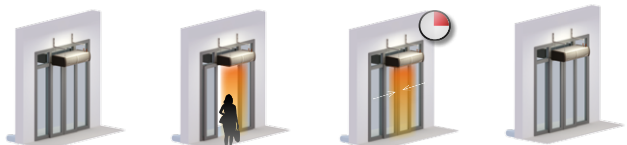
A) Doors are closed - fans are stopped.
