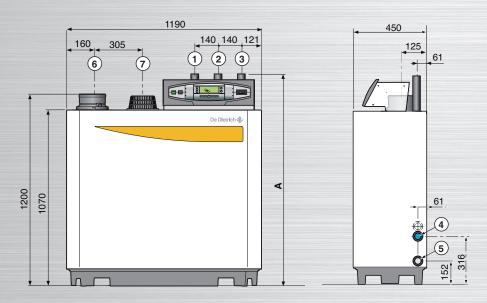
0.54 m² floor space Weight empty = 200 kg / 217 kW I.e. less than 1 kg / kW
